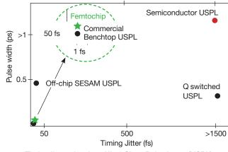
Timing jitter of various Ultra-Short Pulse Laser (USPL) technologies
